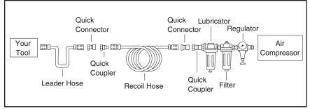
Figure 2. Typical filter and regulator installation order.
